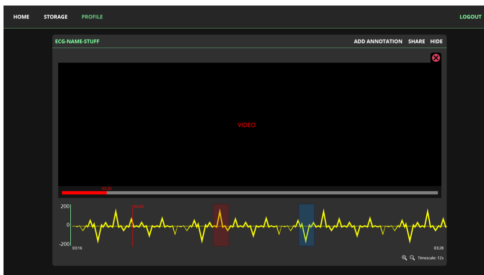
Figure 4.6: Page prototype where the user can visualize the acquisition video itself together with its biosignal data.
