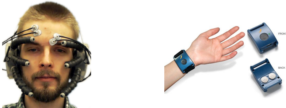
Figure 2.1: Apparatus for BCI. a) Head-mounted measurement device presented by Rantanen et al. [1]. b) The wrist worn Affectiva used by Birjandtalab et al. [2].
