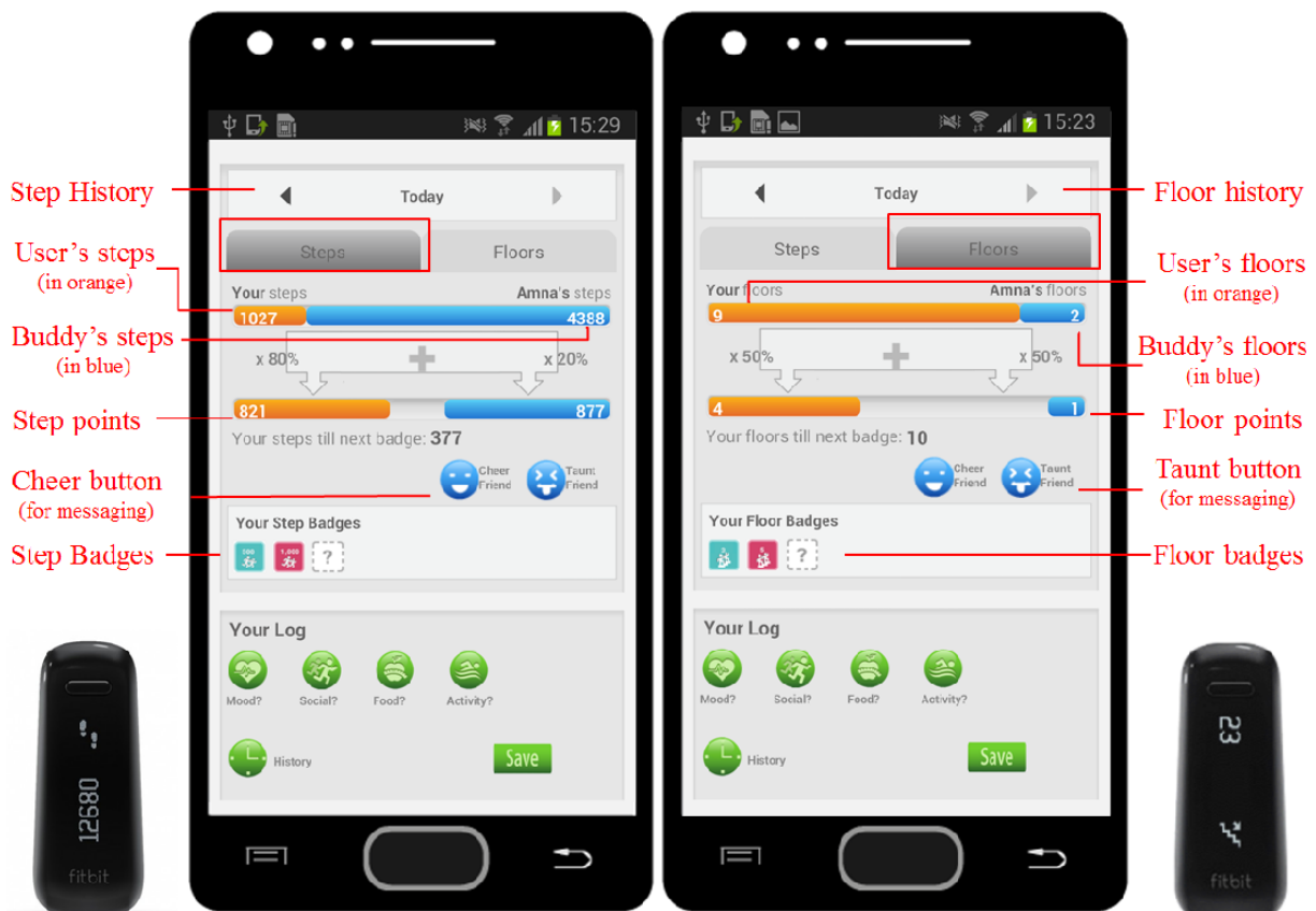
Figure 2.3: Interface of the “HealthyTogether” system [3] for both users, alongside the Fitbit tracker interfaces used.
