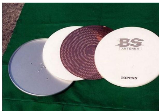
Fig. 1 - Example of a Radial Line Slot Antenna [1]
