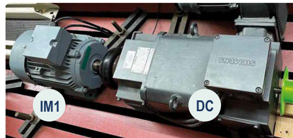
(b) IM1 coupled to a DC machine
