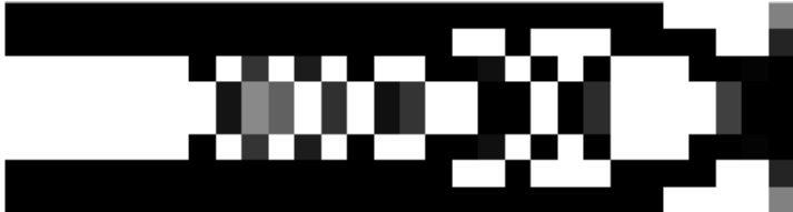
Figure 4.21: Obtained optimal solution for maximum buckling strength of the column after 49 iterations.
