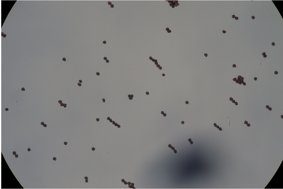
Figure 5.15: Pictures of particles under influence of a magnetic field.
