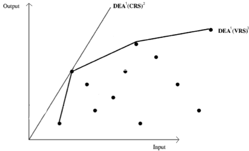
Figure 4.2: Data Envelopment Analysis productivity frontiers assuming Constant Returns to Scale and Variable Returns to Scale (each dot represents a Decision Making Unit).
