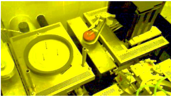
Heidelberg Instruments Direct Write Laser Lithography System: Direct write lithography system HeCd laser (λ=442 nm (g-line) / write lens NA= 0.85) => critical dimensions down to 0.8 µm. System works with mask designs in GDS2 format.
