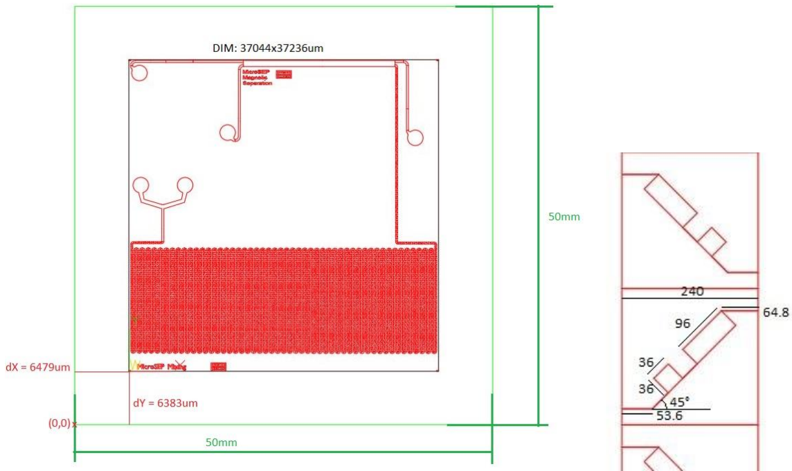
Figure 52- CAD file of the first design of the microfluidic device produced, on the right zoom on channel and obstacles. (all measures are in \mu\text{m} if not differently specified)
