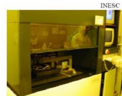
Heidelberg Instruments Direct Write Laser Lithography System: Direct write lithography system HeCd laser (λ=442 nm (g-line) / write lens NA= 0.85) => critical dimensions down to 0.8 µm. System works with mask designs in GDS2 format.
