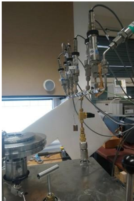
Figure 79 - Structure for holding the pressure transducers connected to the dead weight tester with the pressure transducers connected to the channels for the data acquisition.
