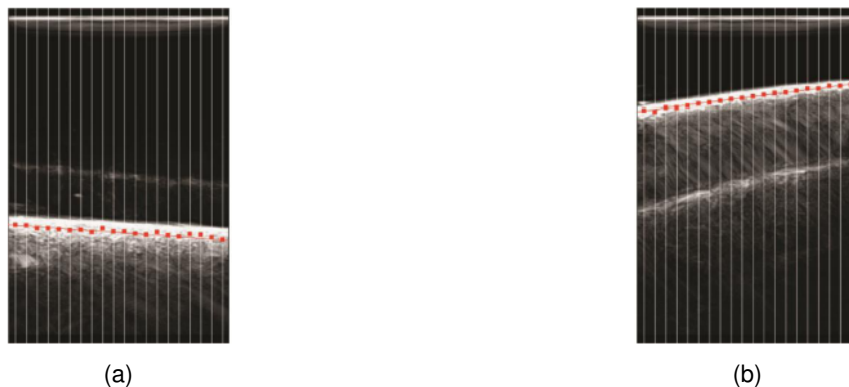
Figure 4.14: Segmented bottom of the tank. In (a) the probe was away from the bottom of the tank while in (b) the probe was closer to the bottom of the tank. (Adapted from [41])
