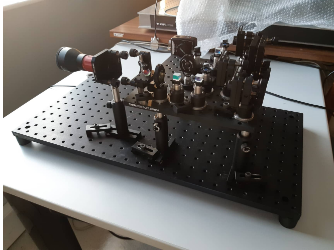
Figure 2.5: Optical setup of the emitter (Alice) used for the BB84 protocol.
