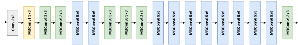
Figure 2.14: Architecture for the baseline EfficientNet-B0 network. Mainly constituted by Mobile Inverted Bottlenecks(MBConv).
