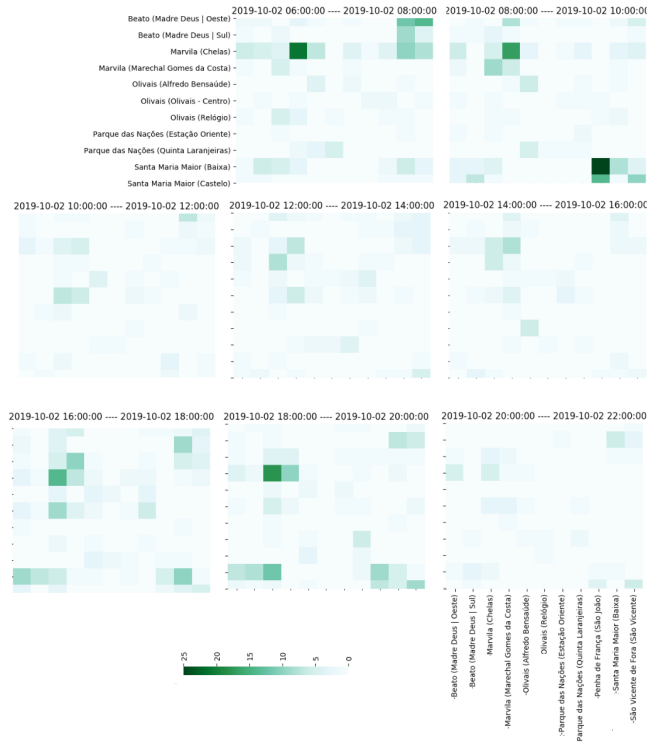
Fig. 10. Matrices with passenger flows in 2-hour periods during the 2nd of October, on route 759, with TAZ granularity
