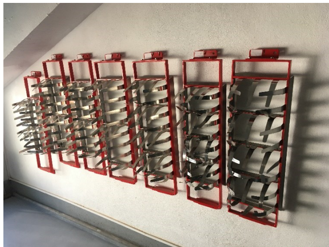
Figure 3 - Placement of brackets on the wall for machine molds
