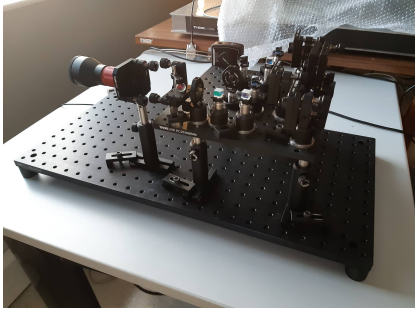
Figure 2: Optical setup of the emitter (Alice) used for the BB84 protocol.
