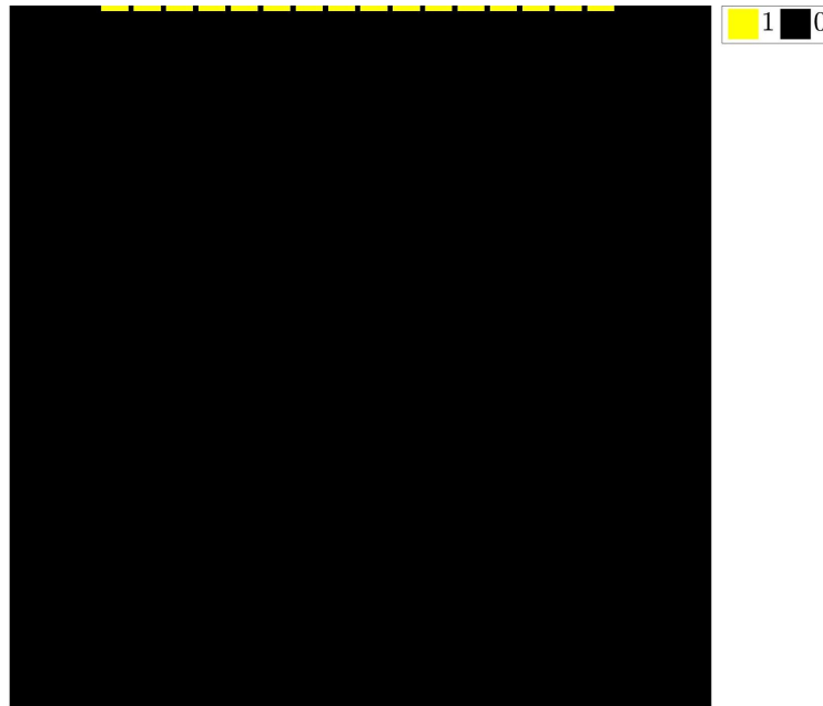
Figure 3.2: Source and sensor binary masks emulating a phased array transducer, where the yellow points represent the active sensor mask. In this case, l_N = 5 , k_N = 1 and N_x = N_z = 128
