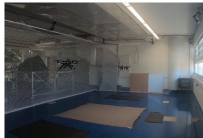
Figure 7: Two drones performing the setpoints tracking test in the ISR Flying Arena.
