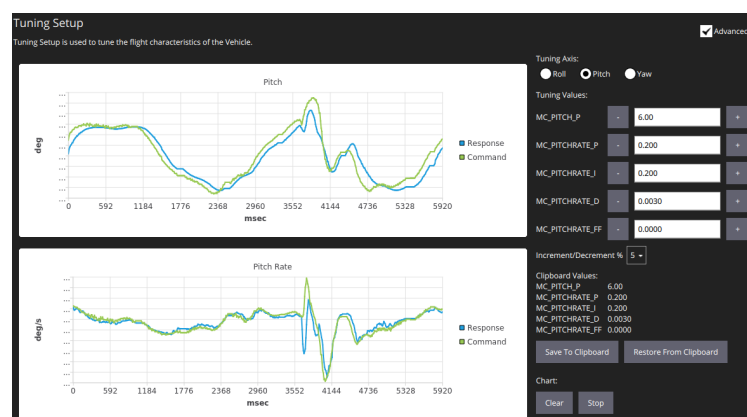
Figure 3.12: PID tuning setup available in the QGroundControl software.
