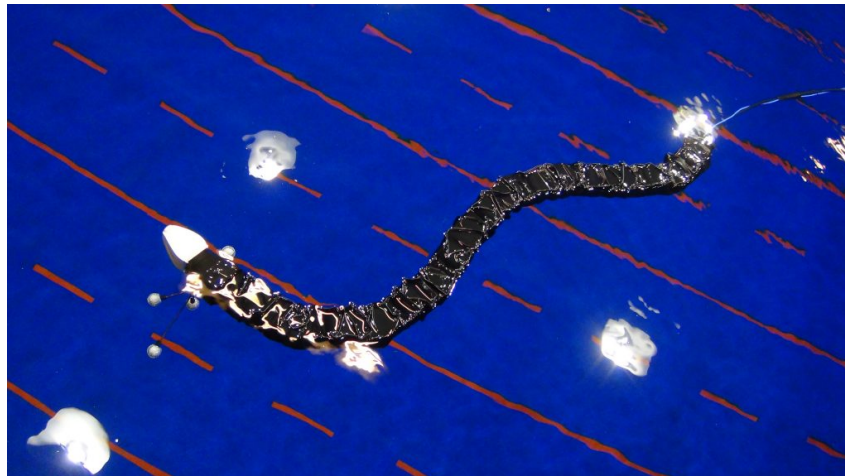
Figure 2.5: Underwater Snake Robot Mamba
