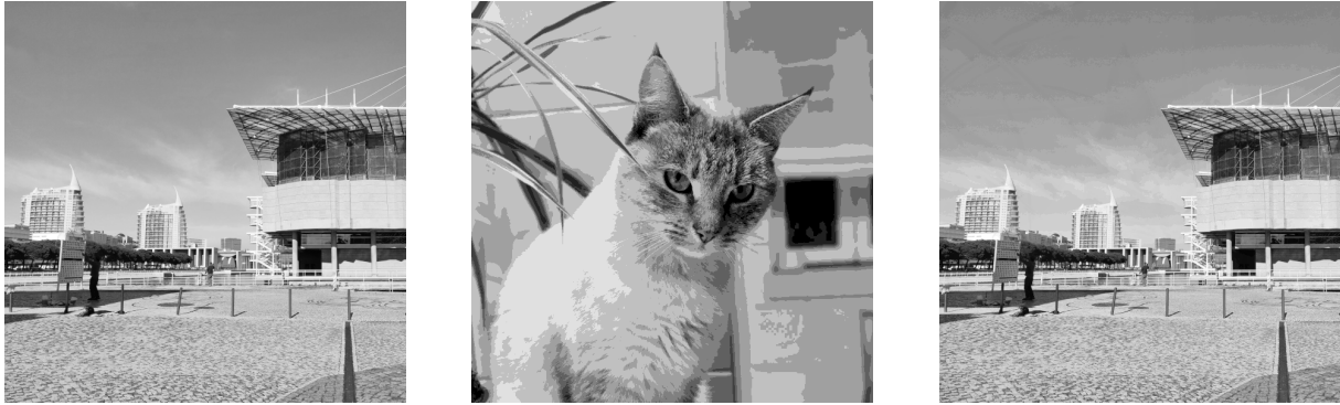
Figure 2.3: Demonstration of an image steganography system, using Stanley's implementation available in [1]. This is an LSB (lowest significant bits) encoding system. The three least significant bits in the pixels of the cover image (left) are replaced with the most significant bits of the payload image's pixels (middle). The resulting image (right) appears largely unchanged except for a slight quality loss and slight noise. These alterations are more obvious in the smoother areas of the image, such as the sky.
