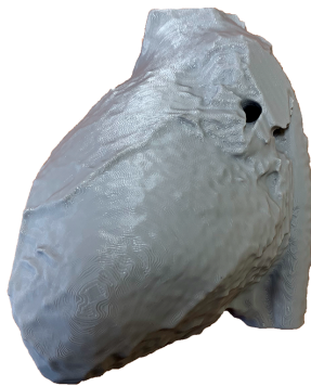
Figure 19: Result of the printing of the left section of the hollow model made with the CT scan of the heart of the patient with ToF. Left view.
