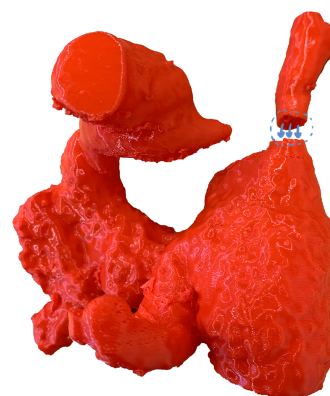
Figure 26: Result of the printing of the right heart segment made with the CT scan of the heart of the patient with ToF. A piece of the superior vena cava fractured and, the blue circle and arrows show where the fragment should be. Posterior view.
