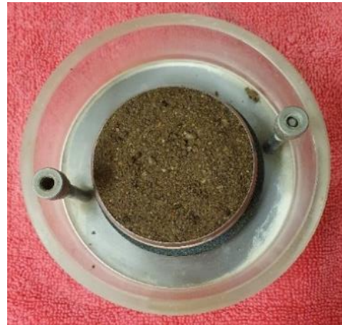
Figure 2 - Treated sample inside the oedometer cell.
