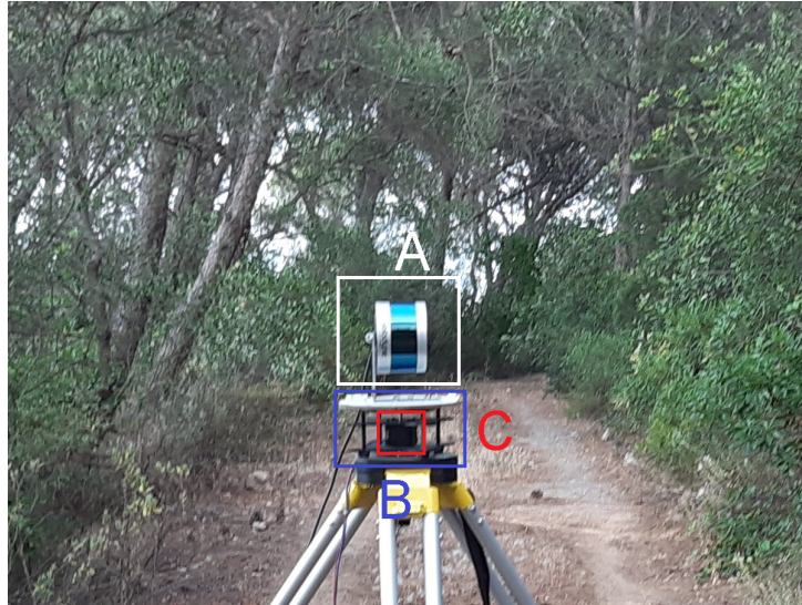
Figure 3.3: Low Cost stationary LiDAR system. This system is composed by the LiDAR sensor (A), a turntable (B) and a step motor (C).
