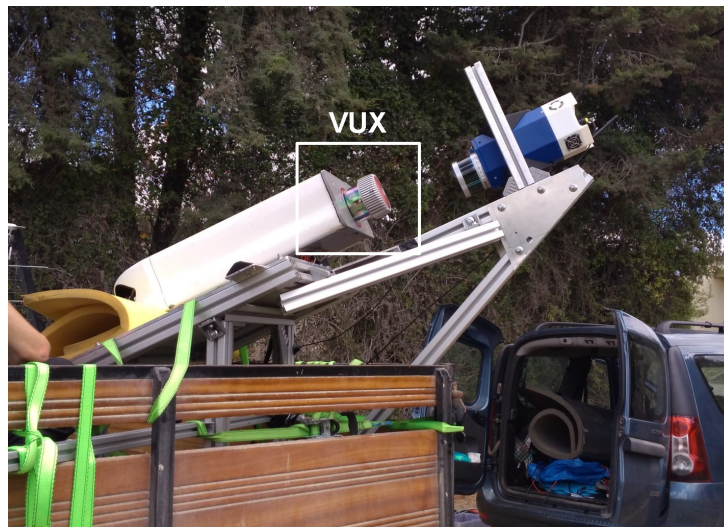
Figure 4.12: MLS implementation using RIEGL VUX-1UAV LiDAR sensor.
