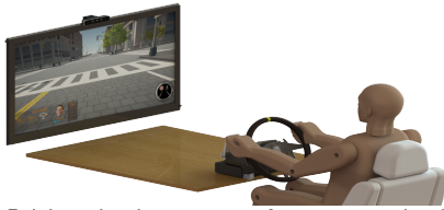
Figure 2: Driving simulator setup: A computer simulated environment is presented in the screen, while the driver controls a vehicle using the pedals and Cardiovheel. The simulator not only integrates the inputs to run the environment, but also aggregates inputs from the wheel movements, CardioWheel sensor, and intel realsense camera to a database.
