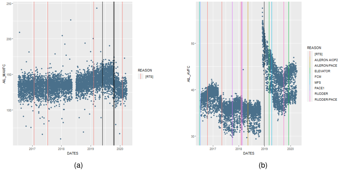
Figure 3.9: Examples of aileron force feature correlation to pilot complaints on control stiffness
