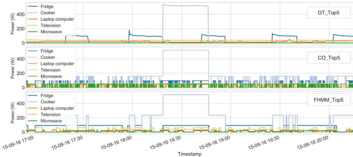
Figure 3.4 DRED: The five most consuming appliances' disaggregation
