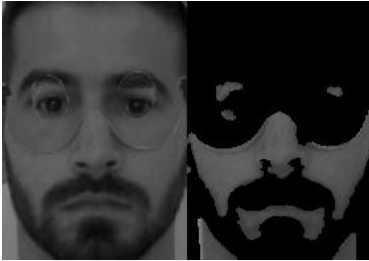
Fig. 7. Original image (left) and binary map (map), after applying the proposed skin detector.
