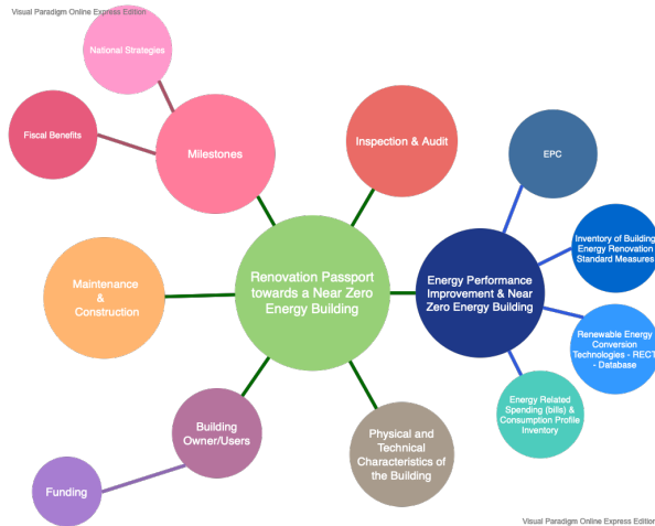
Figure 4: Components of the Renovation Passport, with their respective input databases, and connections between them.
