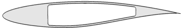
Figure 5: Graphical representation of the RAE 2822 case of study complemented with the aerofoil and wing-box skins.
