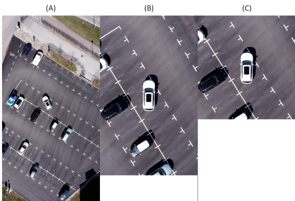
Figure 1: Images of the same frame after different rectifying steps. (A) - Original frame; (B) - Frame after alignment and centring; (C)- Frame after cropping.
