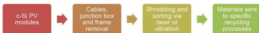
Figure 3.7. Summary of PV cycle recycling process for c-Si modules (Lunardi et al., 2018)
