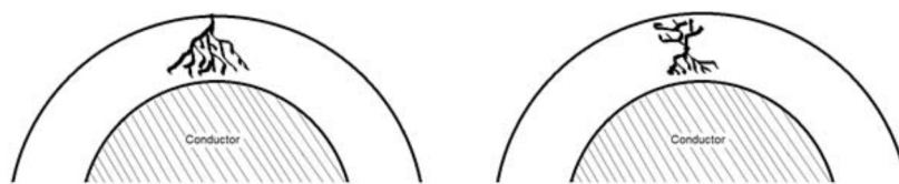
Figure 2.9: Vented Tree (Left) and Bow-Tie Tree (Right) (From A Hybrid High Frequency Pulse and Pattern Recognition Method for Water Tree Detection in Long Distance Underground Cables [2])
