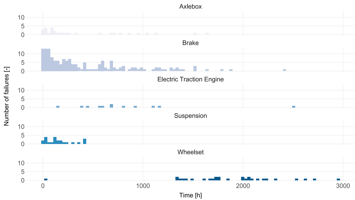
Figure B.3 – Scenario 3 a) total histogram covering the number of failures of the system regarding each subsystem failure and b) each subsystem histogram decomposed
