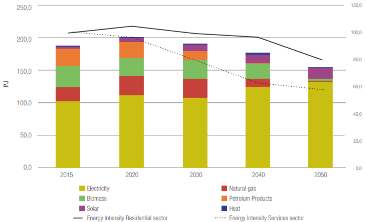
Figure 6. Evolution of final energy consumption [PJ] and energy intensity in buildings (residential and services) [15]
