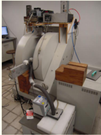
Figure 2.4: Electromagnet used for medium field measurements.
