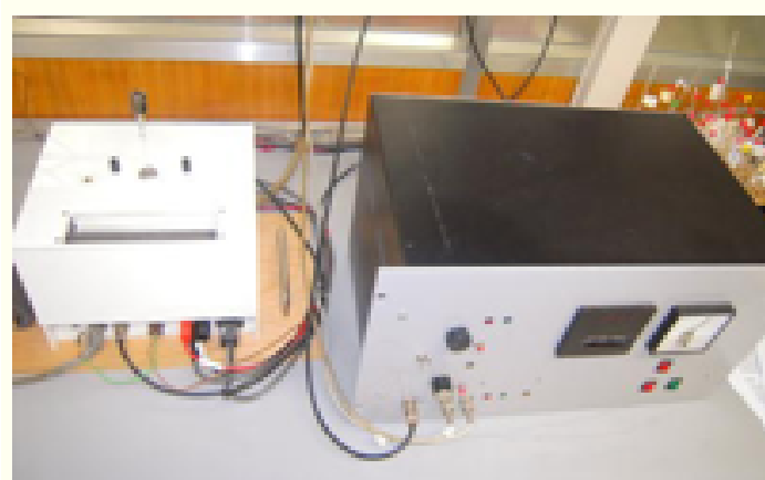
Figure 2.3: FFC spectrometer used for low field measurements.
