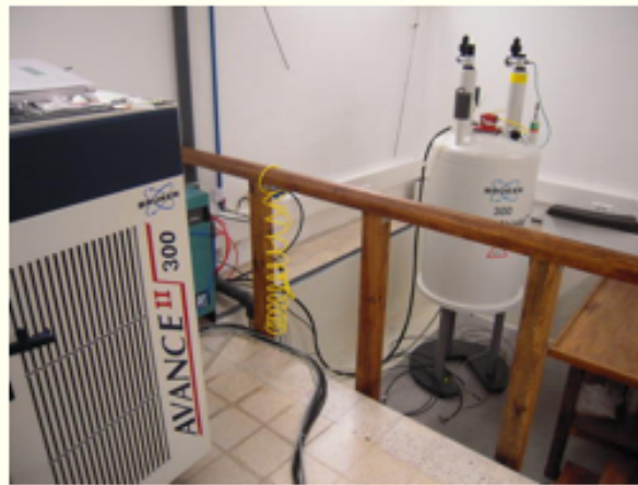
Figure 2.5: Superconducting magnet used for B = 7T .
