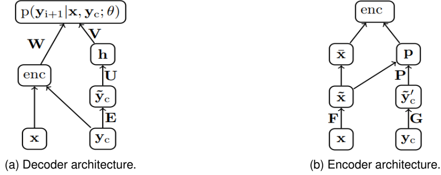
Figure 2.11: Illustration for the basic encoder-decoder architecture for sequence-to-sequence transduction, adapted from Rush et al. [2015]
