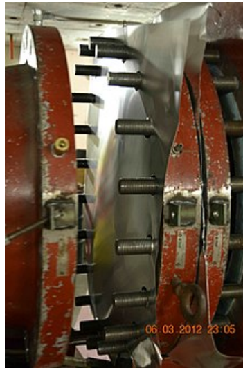
Figure 2.2: Example of how an aluminum diaphragm is clamped in a shock tube, photo taken by Achim Hering.
