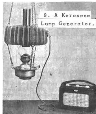
Figure 1.7: The use of a TEG incorporated in a kerosene lamp to power a small radio was idealized by Soviets in the beginning of cold war; those were useful in rural places of Siberia and China, not yet electrified.
