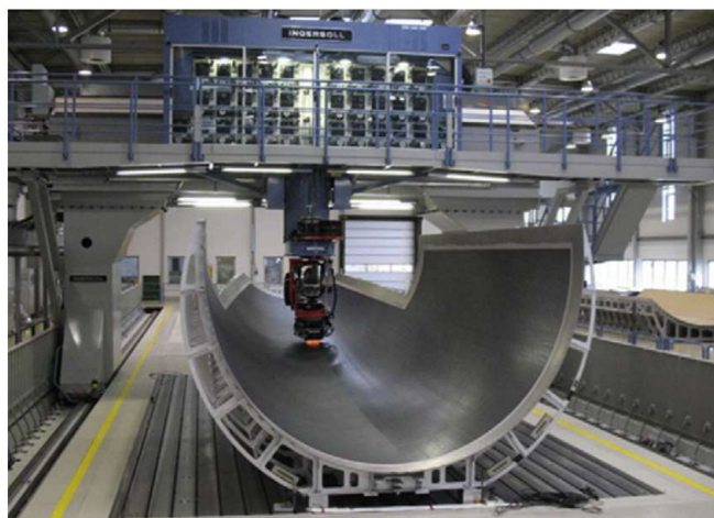
Figure 7 - AFP gantry structure with tow holder on top of the horizontal column, laminating over an open mold [29].
