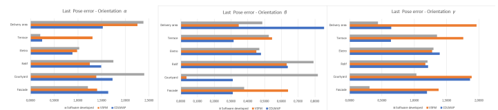
Fig. 15. Graphic of the error variation according to each of the Euler angles. a) Graphic of Yaw error on the last pose \alpha . b) Graphic of pitch error on the last pose \beta . c) Graphic of roll error on the last pose \gamma .
