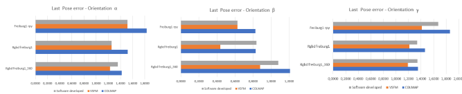
Fig. 18. Graphic of all rotation errors in the last pose of the camera. a) Graphic of the last pose yaw error \alpha . b) Graphic of the last pose pitch error \beta . c) Graphic of the last pose roll error \gamma .
