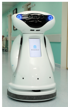
Figure 6: MONarCH Robot – the social robot used in the experiments
