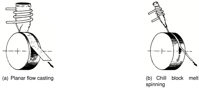
Figure 2.10: Preparation of soft magnetic ribbons by means of rapid quenching from the melt [17].
