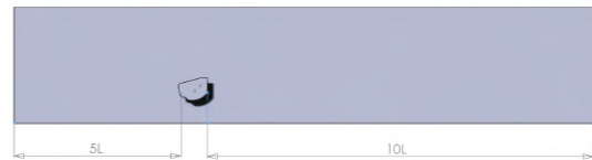
Figure 5: Domain used in the CFD simulations.
