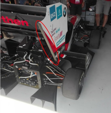
Figure 3: Gurney flap on an endplate of a FS car.
