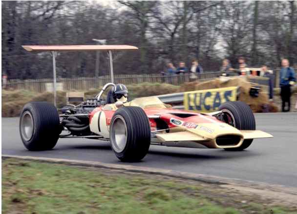
Figure 1.1: Lotus 49B Formula 1 racecar. While it debuted in 1967, the wings were only introduced mid-way through 1968. Given a series of accidents due to inappropriate mounting structures and adjustable angles of attack, they were promptly banned [3].
