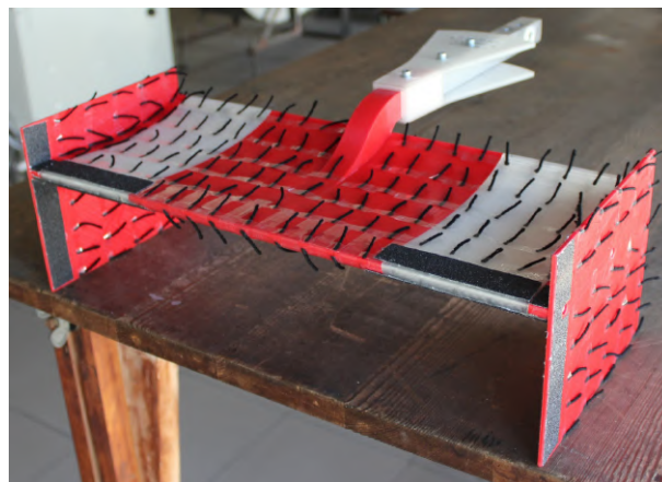
Figure 5.6: Wing model with woolen threads and sand paper as used in the last test run for the yaw angles.
