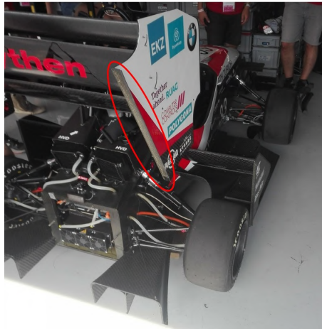
Figure 1.16: Gurney flap on an endplate of a FS car.
