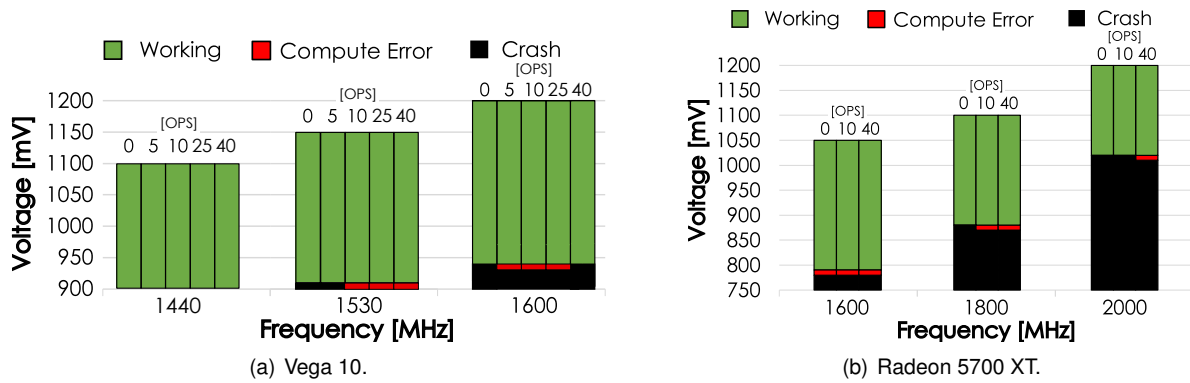
Figure 3.4: Core domain - Shared Memory - Usable voltage range for each frequency configuration with varying shared memory stress ( OPS parameter).
