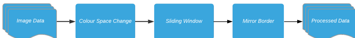
Figure 3.3: Pre Processing operations from the raw image to the processed network's input
