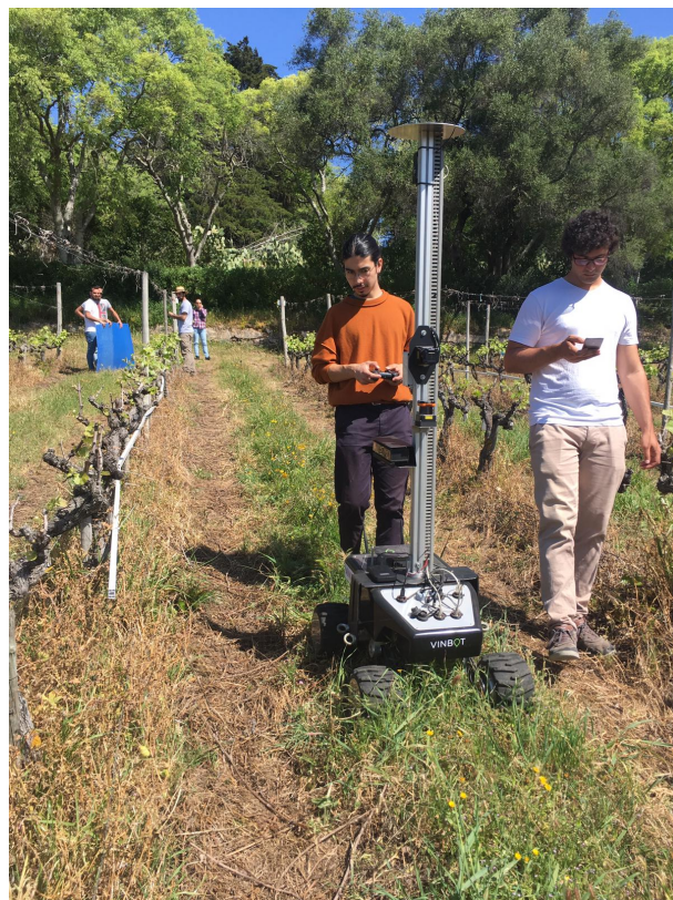
Figure 3.1: Vinbot robot driven by the Vinbot team, collecting data from the earlier stages of the vines development at the red variety vineyard of Instituto Superior de Agronomia (ISA)
