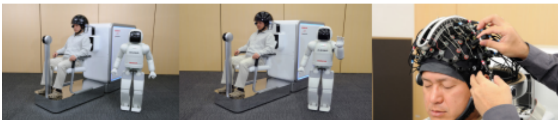
Figure 2.3: ASIMO humanoid robot replicating human body movements that are derived from the analysis of the user's thought process. [14]
