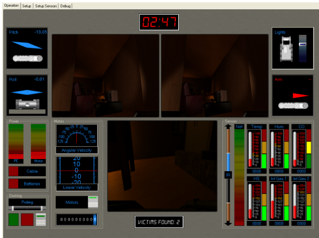
Figure 6.7: View of the interface displayed during the stress task, showing a timer in the top and a victim counter in the bottom
