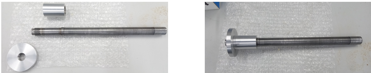
Figure 3.10: (a) Drawbar disassembled and (b) assembled
