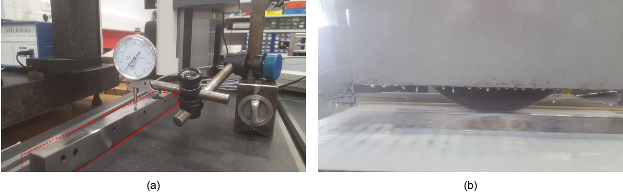
Figure 3.7: (a) Master rail (circled in red): checking for flatness (b) Grinding the master rail
