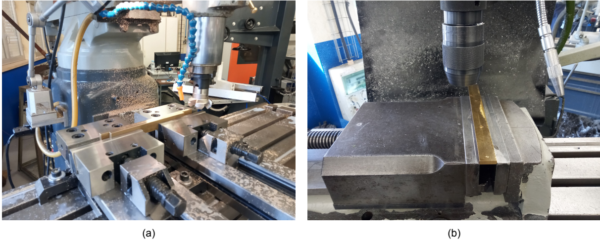
Figure 3.8: (a) Milling of the brass gibs (b) Locating hole drilling
