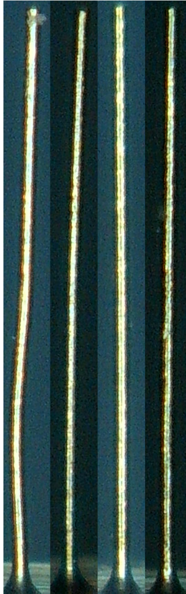
Figure A.10: Two most left: a_p = 0.5 mm, f = 0.005 mm/rev. to f = 0.010 mm/rev.; Two most right, a_p = 0.9 mm, f = 0.005 mm/rev. to f = 0.010 mm/rev.
