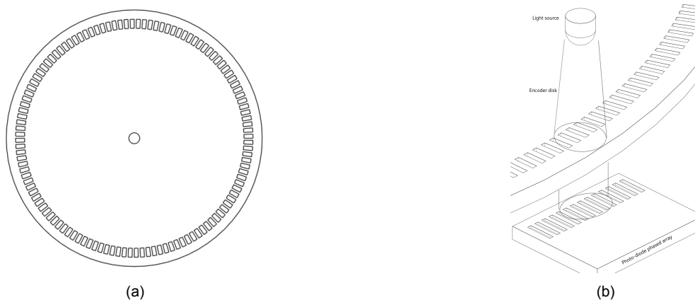
Figure 2.9: (a) Incremental encoder disk, no index track (b) Typical incremental encoder assembly
