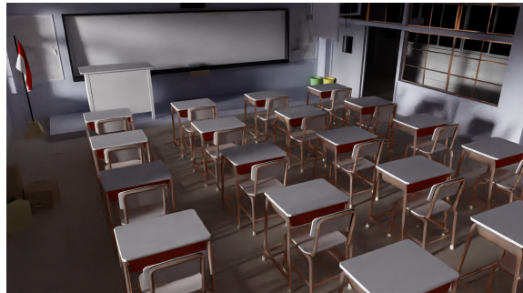
Figure 8: "Japanese Classroom" - Path Tracing with Denoising - 8 Total Accumulated Samples - Rendered in 16 milliseconds + 14.5 milliseconds of denoising
