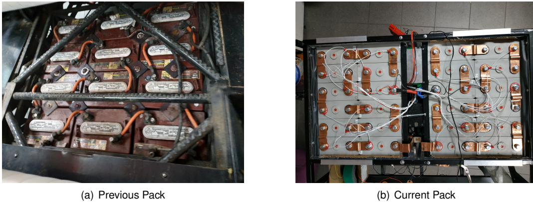
Figure 3.18: Pictures of the two battery packs used in the e-tuk Limo GT .
