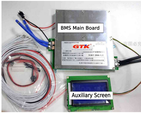
Figure 3.4: Photo of a similar BMS to the one used in the vehicle.
